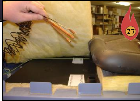
Install 3 Control Panel Sensors into Port #23. Make sure they are pushed all the way to bottom.
