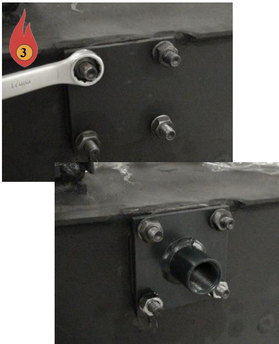
Remove Coil Plate on Either the Right or Left Side and Install Pressure Relief Valve Flange
