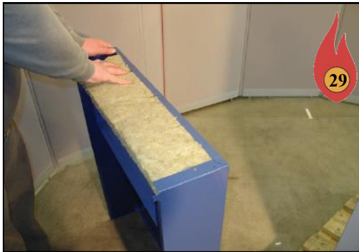
Install Insulation on back of top panel.
