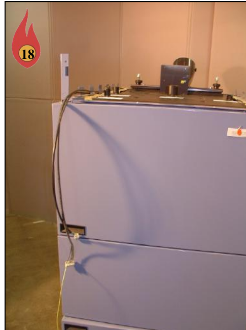
Leave Fan Wire Hanging in Front of Front Panel
