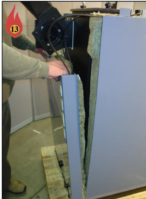
Place Rear Panel into Place (Electrical box not shown)
