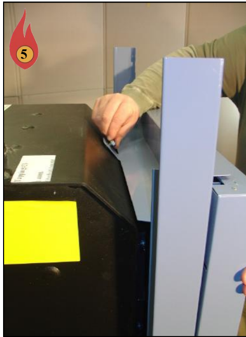
Install Front Panel Mounting Bolt and Washer
