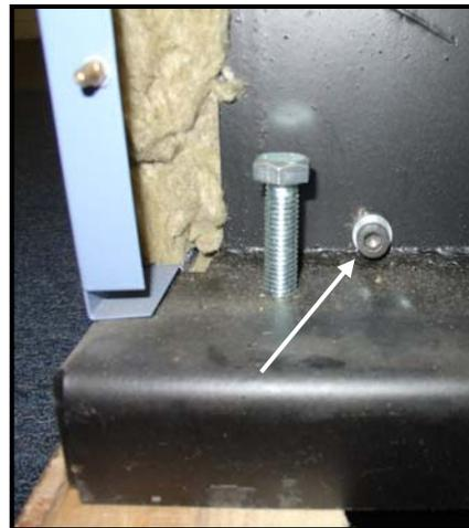
Fig. 5.2 Drain Plug Models 1.5 and 4.0
